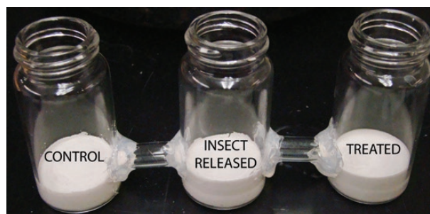
Fig. 1. Choice bioassay setup using three scintillation vials joined by glass tubes. Holes were made in the scintillation vials with a DeWalt 6.4-mm diamond drill bit. One adult female was released in the central arena and had a choice of going to the control berry or to a berry treated with 80 \mu\text{g}/\mu\text{l} ( E,E )- \alpha -farnesene.
